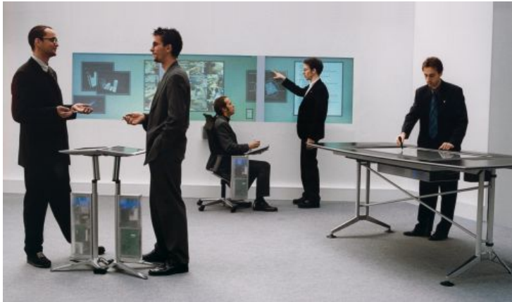
Fig. 1. Examples of Roomware components: DynaWall, InteracTable, CommChair, ConnecTables
